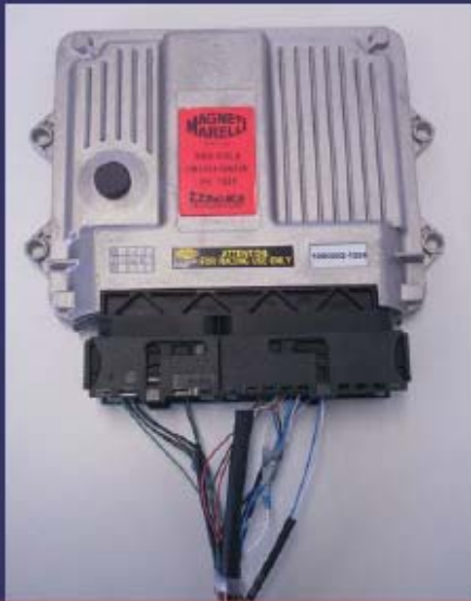
Electronic Control Unit
